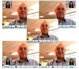
The icon on the PIP softkey indicates where the PIP window will appear when you next press the PIP softkey.
